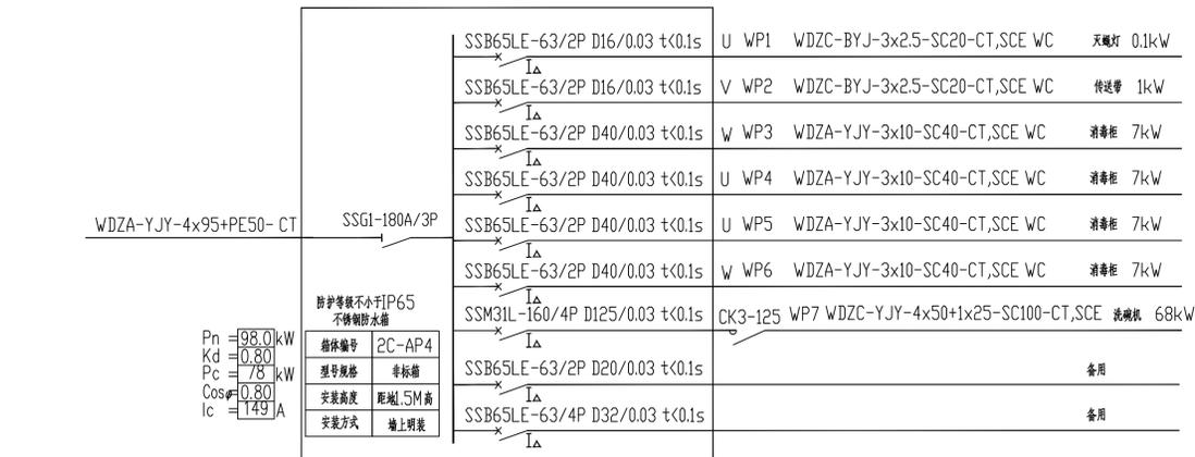
Technical specifications for the second diagram: Pn=98.0kW, Kd=0.80, Pc=78kW, Cosφ=0.80, Ic=149A.
