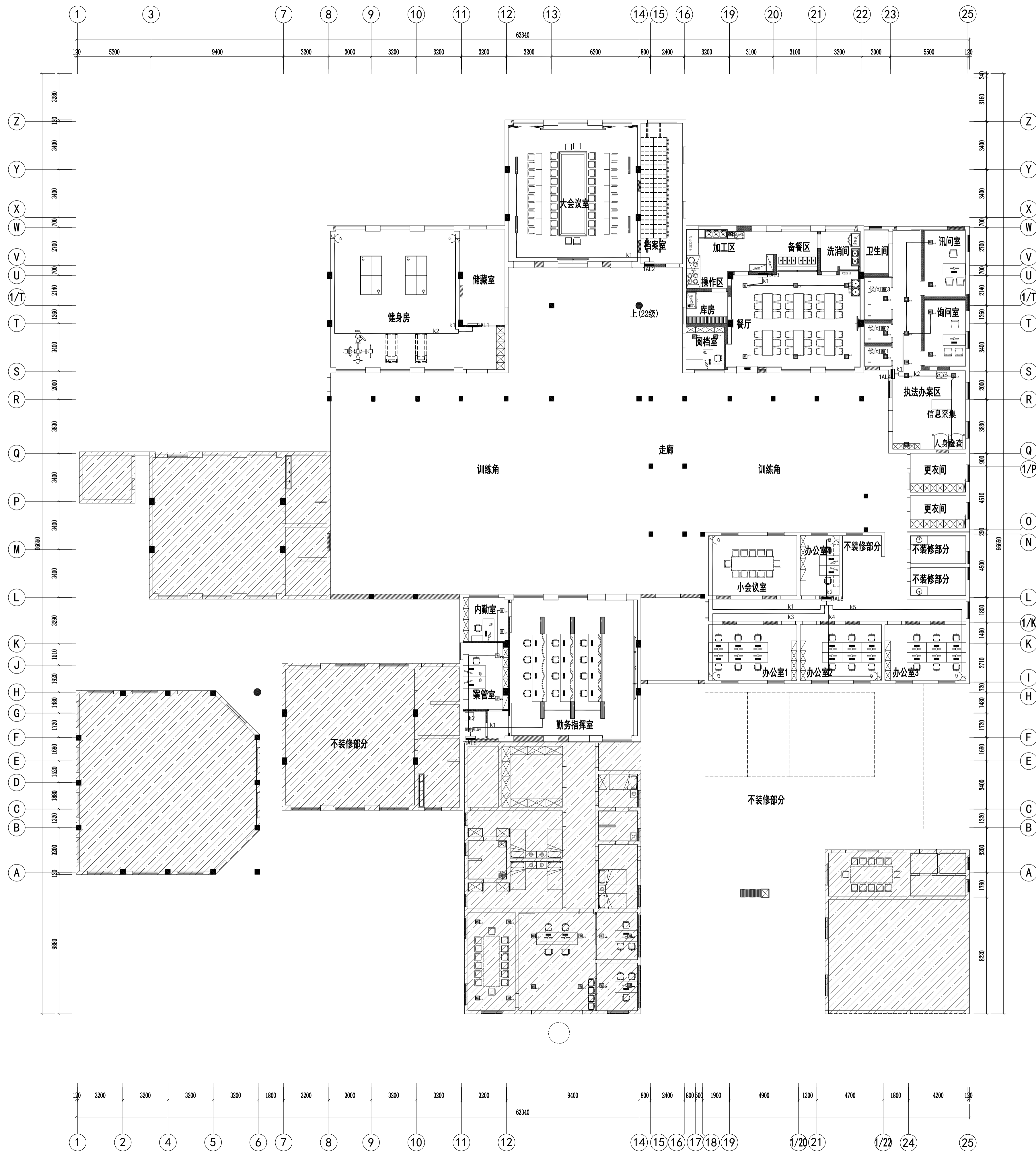
1F REFLECTED LIGHT CEILING PLAN 一层总顶面灯具放线图 SCALE: 1/150
