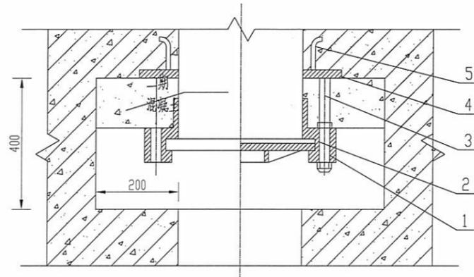
1-门框和导轨;2-止水密封条;3-地脚螺栓和调整螺母;
